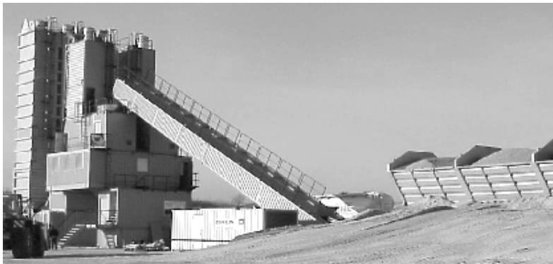
Fig. 4: Newly developed concrete batch mixer which fits completely in seaworthy ISO containers, capacity 240 m 3 per hour
