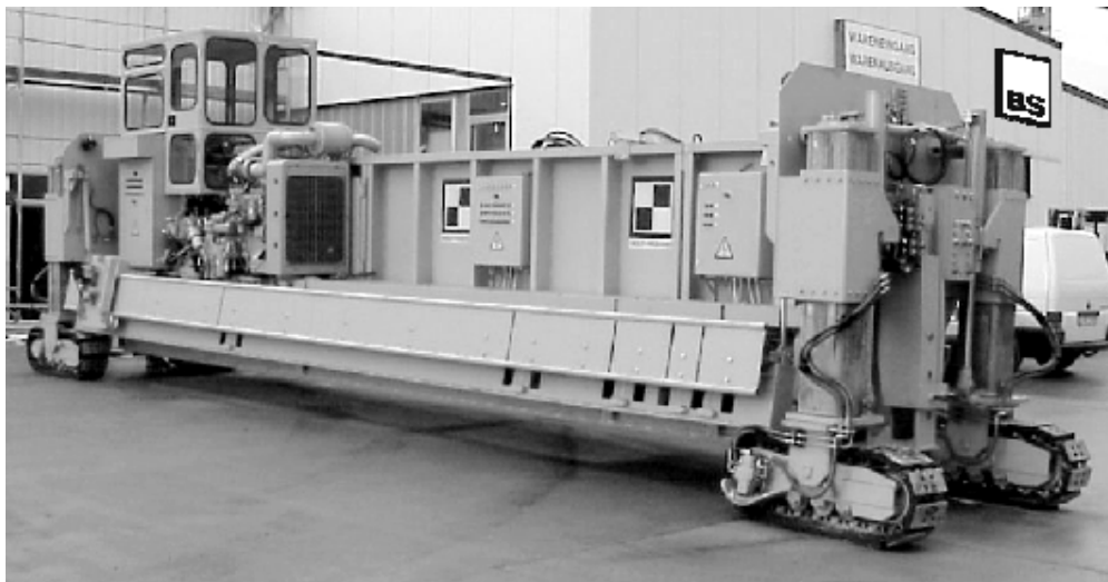
Fig. 5: Newly developed Slipform paver which can be transported completely in seaworthy ISO containers without the need for much alteration work – ready for driving in an ISO container
