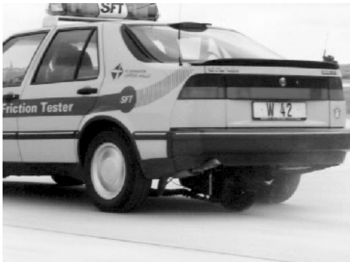
Fig. 13: The concrete pavement for the aircraft movement areas of the Munich airport still provides good skidding resistance; Saab Friction Testers are used for testing the skidding resistance of aircraft movement areas in Germany
